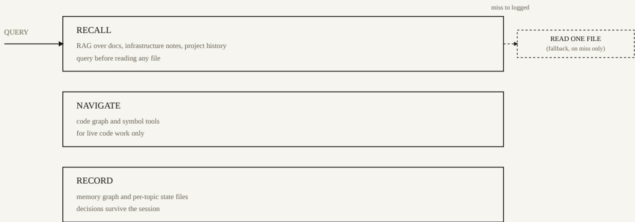
Figure 4. A query hits recall first and only falls through to a single file read on a miss, while navigate and record serve code work and durable state on their own tracks.
